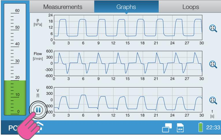
Figure 52: Monitoring screen (freeze graphs)
