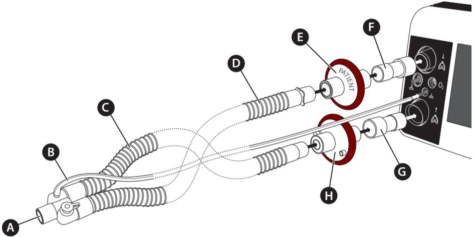
**A** Patient side connection **B** Pressure measuring tube **C** Expiration tube
