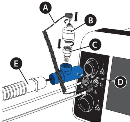
**A** Connecting line   **B** FiO<sub>2</sub> sensor   **C** Housing gas duct
