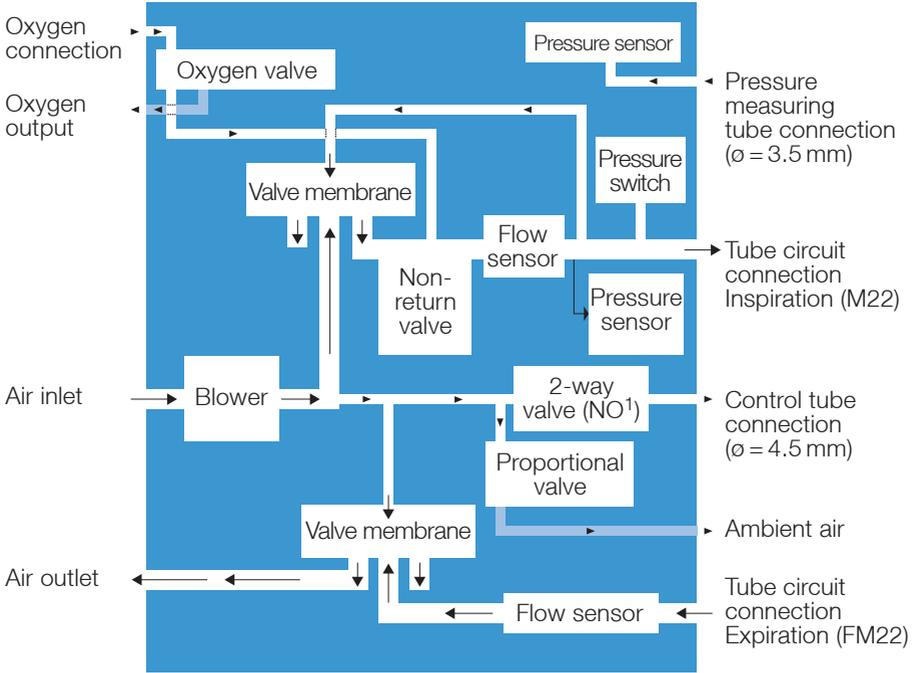
Figure 77: Pneumatic block diagram
