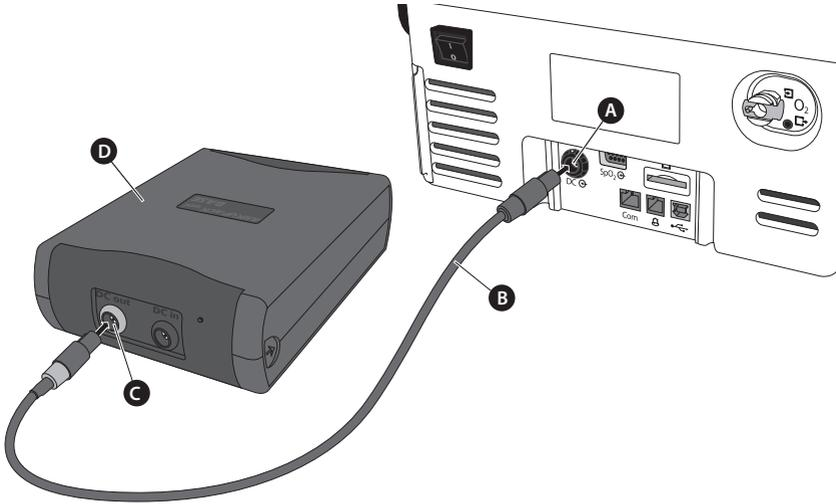
**A** DC port   **B** DC cable for ventilation   **C** DC out (device connection )
