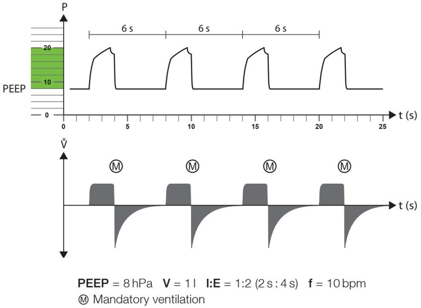
Figure 39: VCV mode diagram
