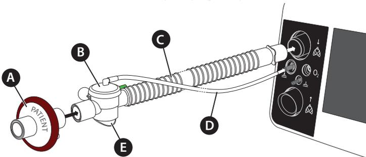
**A** Bacterial filter   **B** Expiration valve   **C** Ventilation tube   **E** Control tube
