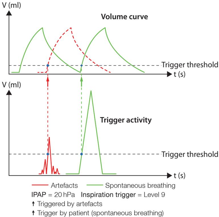
Figure 44: Inspiration trigger without SMART Function
