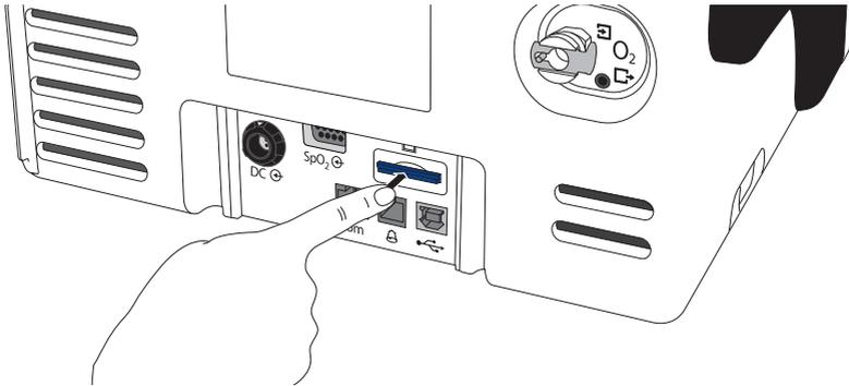
Figure 26: Removing SD card
