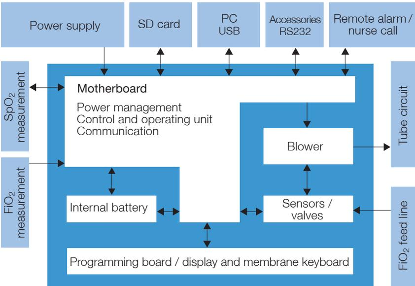
Figure 76: Block diagram for the device
