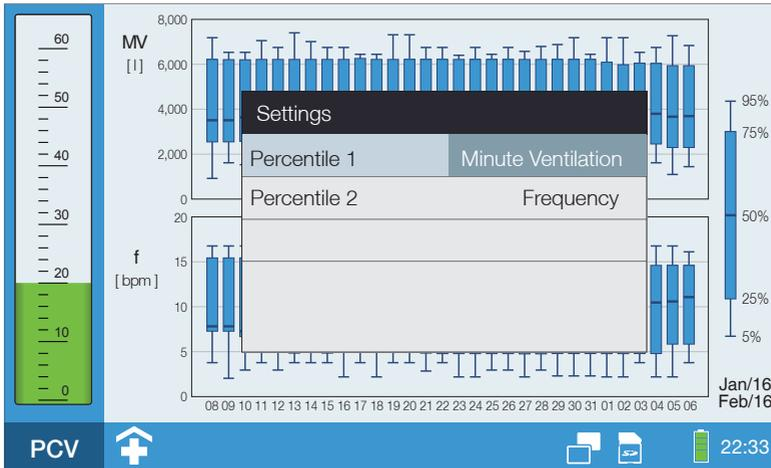
Figure 64: Statistics screen (2 ventilation parameter)
