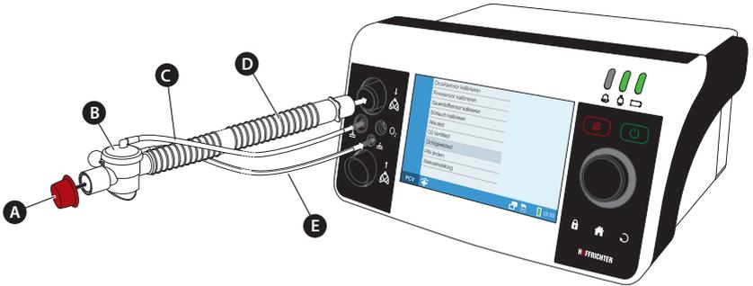
A End cap (supplied with the tube circuit) B Expiration valve
