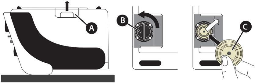
**A** Bottom flap **B** Valve cover **C** Valve membrane
