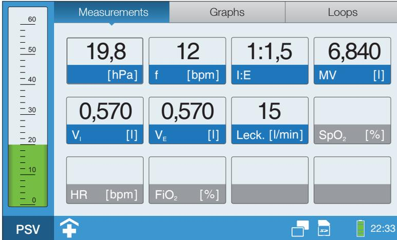
2. Navigate to the measured value box that you would like to configure by turning the MFK. Press the MFK to activate the measured value box.
