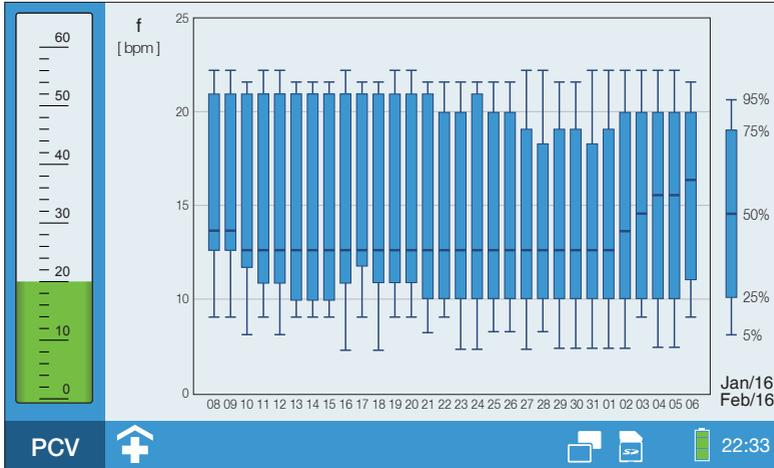
Figure 63: Statistics screen (1 ventilation parameter)
