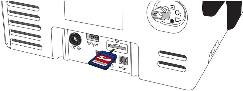
Figure 24: Inserting SD card
