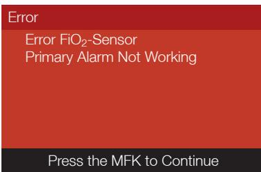
To hide the error list, press the MFK. The default parameters are not loaded. If ventilation is active, it continues to run with the user-defined settings. However, the device can no longer be operated.
