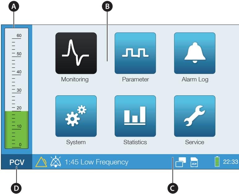
**A** Pressure bar (during running ventilation)   **B** Screen content
