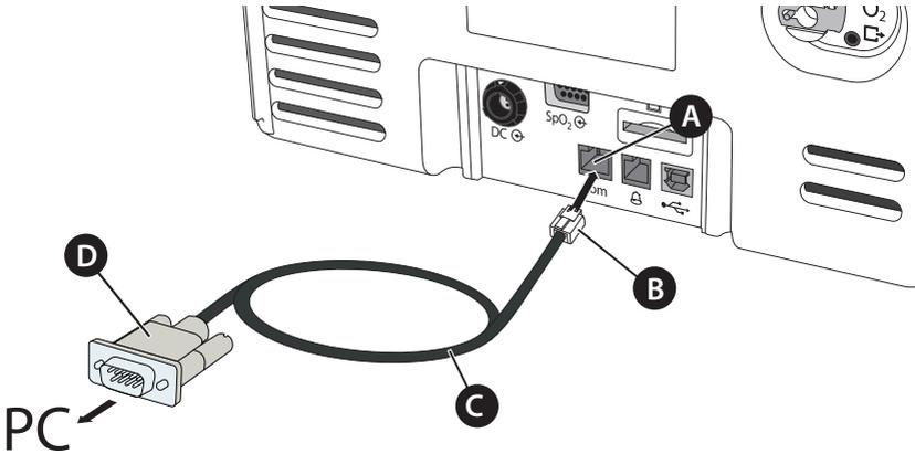
**A** USB interface   **B** USB type B plug   **C** USB cable (PC cable)   **D** USB type A plug
