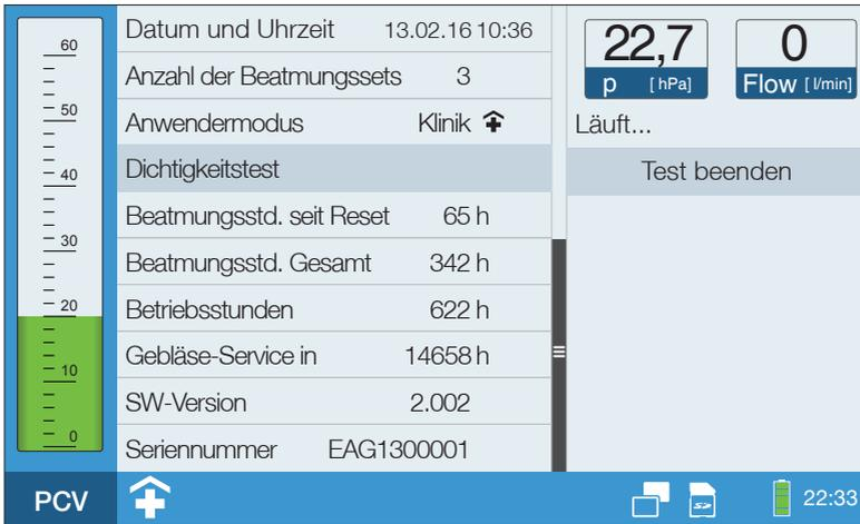
The pressure is gradually increased to the maximum pressure by the device. Observe the flow value. If the flow value exceeds 5 l/min during the tightness check, there is a leak in the tube circuit. In that case, check the entire circuit for leaks in tubes and at tube connections. As long as the flow remains under 5 l/min the tightness check is positive. Press the MFK to complete the test.
