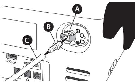
**A** Oxygen connection   **B** Oxygen connection adapter, straight
