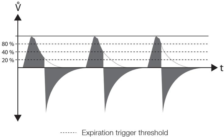
Figure 43: Flow trigger (setting a percentage value)
