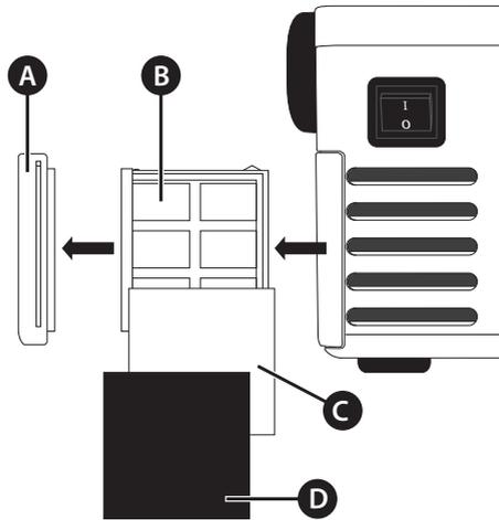
**A** Filter frame cover   **B** Filter cassette   **C** Fine filter (white)
