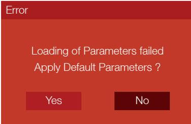
If the boot process is initialized during ventilation, ventilation continues. However, the device can no longer be operated. The user now has the following options:
