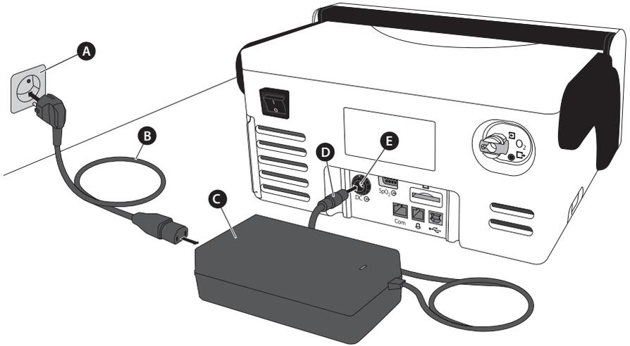
**A** Power socket **B** Mains cable **C** Power supply **D** Power supply plug
