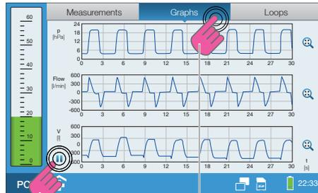
Freeze real-time curve on the monitoring screen    Select tab
