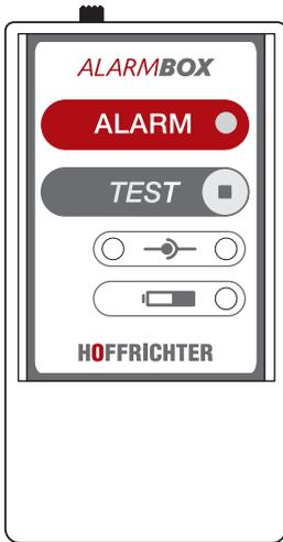
Alarms can be forwarded by using a nurse call or the optionally available alarm box. This allows even better monitoring of the device at the home or clinic. The use of the remote alarm box or a nurse call is especially recommended when several ventilators are used in one room, as this allows the device generating the alarm to be easily identified. The alarms will be forwarded without delay to the nurse call or the alarm box.
