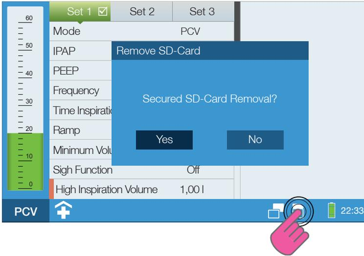
Figure 25: Removing the SD card safely
