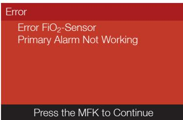
When the MFK is pressed, the default parameters are subsequently loaded, i.e., the device is reset to the factory settings. If ventilation is active, it continues to run with the factory settings. The device is again fully operational.
