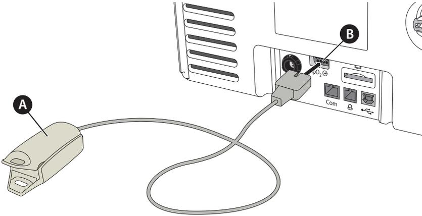
**A** SpO<sub>2</sub> finger clip sensor    **B** SpO<sub>2</sub> sensor connection
