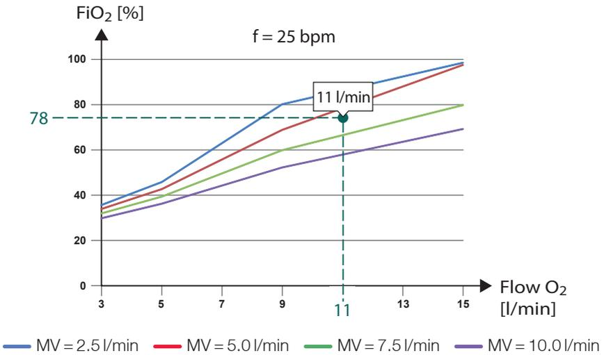
At an oxygen flow rate of 11 l/min and a minute ventilation of approximately 6 l/min, an oxygen concentration of approximately 78 % can be reached.
